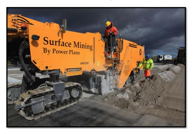
Specially adapted Planing Machines are used for surface mining method of extracting minerals on the surface of the Earth or removing manmade surfaces which are too hard to mill with a conventional planer.
